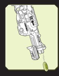
Point the blaster at the ground. The jammed disc will fall out.
